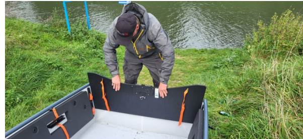
4. Position the transom plate and 5. Secure the transom's cam buckles
