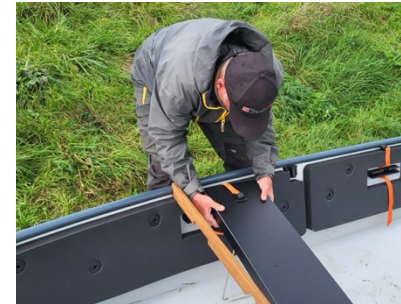
1. Position the middle bench first. make sure the legs end up well in the corners
