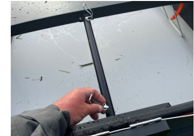
7. Place the tube between the rear seat and transom. Secure it with the clips provided
