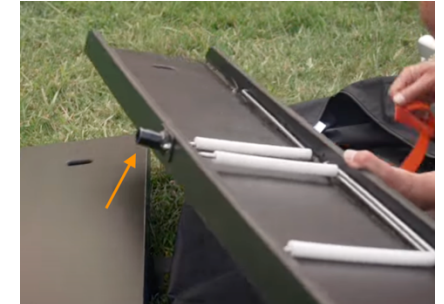
Note: the rear bench has a connector which needs to face the transom
