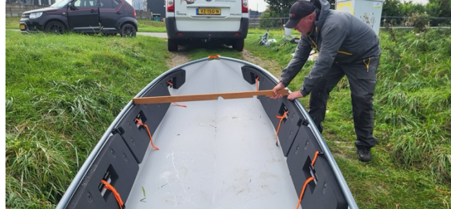
2. Manually open the hull and fix the opened hull with the extension stick provided
