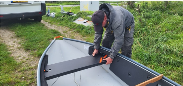
6. Position the back bench next and the front bench last.
